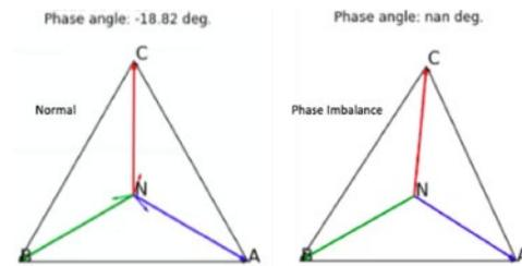
Besides the data-based anomaly detection, APM360 also uses physics-based models to monitor individual devices as well as switchboards. Imbalances in three-phase voltages and currents can be monitored using algorithms in the **APM360 Model Library** for calculating the negative-sequence and zero-sequence voltage and current vectors. These can be used to warn of imbalances at the device (e.g., PQM) level as well as at the switchboard level.
