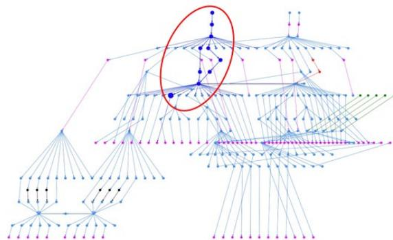
results from individual systems are merged and network analysis algorithms used to “collapse” interrelated alerts from multiple systems into a single alert with probability scores assigned to devices most likely to be the source of the problem.
