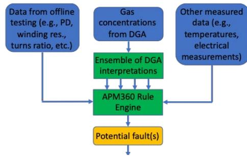
In addition, the FMEA template can be customised and fine-tuned with data, if available, from historical offline testing (e.g., PD, winding resistance, turns ratio, leakage reactance, SFRA, etc.).
